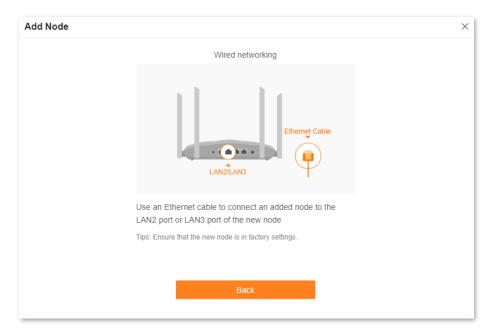
If the LED indicator of new node lights solid on and the new node is displayed in **Network Topology**, the node is added successfully.
