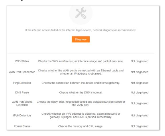
**Step 4** Check the diagnosis result and click **Optimize** to rectify the faults.
